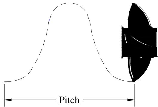
Diameter and pitch are the two basic dimensions of a propeller. Diameter is the distance across the circle made by the blade tips as the propeller rotates. Pitch is the theoretical (not accounting for slippage) forward distance the propeller would move in one revolution. An example of a propeller dimension would be 14 X 17 for a propeller having a diameter of 14" and a pitch of 17".
